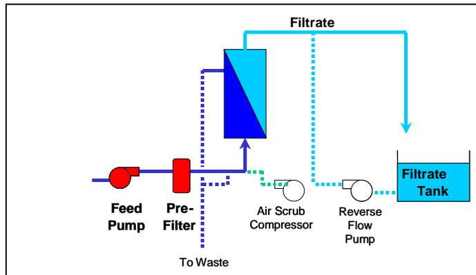
The system remains in filtration until the unit has filtered a pre-set quantity of filtrate. At this point a backwash is initiated. There is also a timer that runs in parallel that can also initiate the backwash sequence.
